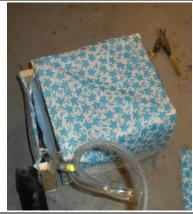
Attach the free end of the hose to the base of an elevated bucket. As the bucket is filled with water, the water will trickle into the cavities, mositening the charcoal and cloth material.
