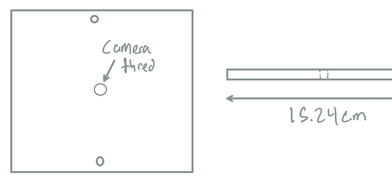
Bolts for belt have to be in line so the don't Create a moment about the camera thread - this will allow plate to slide on rails smoothing will less friction.
