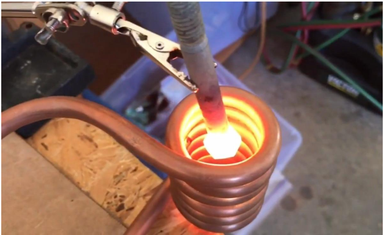
Figure 1: A workpiece being heated by an induction heater
