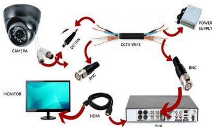
Figure 2-18 (left): Proseses needed to connect place an analog camera (Arsh, 2018).
