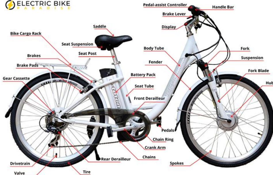
Figure 2-11: Anatomy of an e-bike (Electric Bike Paradise, 2019)
